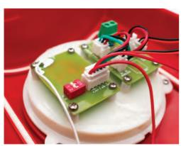
7. Once all units have been paired, remove the batteries from every alarm and change the "S1" position on the master alarm to "Off".
