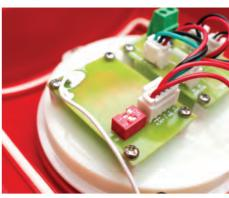
With the batteries unplugged turn the "S1" switch on the master alarm to "ON"
