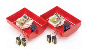
6. Only switch the position of "S1" on the master alarm. Install the batteries into other units you wish to connect, the unit will start to beep intermittently. This indicates the pairing process is complete.
